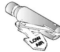
Low Pressure Warning
